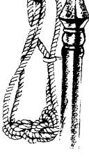
b. Pass loose ends of C&T through and over loop above screw eye.
